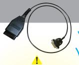
When using the EOBD cable (GO2114) the SPECTRUM pro must NOT be connected to any power
